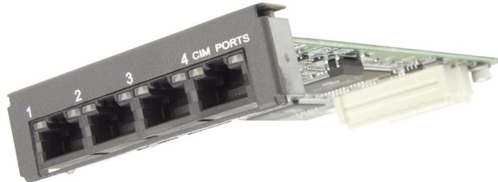
The Quad CIM is used in the CX Controllers, CXi Controllers, and MXe Controllers when further ASU's need to be connected to the controller. A single Quad CIM can be installed into a CX Controller and CXi Controller, but when the Quad CIM is installed into the CX Controller and CXi Controller, only the first three ports can connect to ASU's. The fourth port will be inactive.
