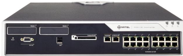
The CX Controller and CXi Controller are typically used for small business solutions, or in a branch office, and can support a maximum of 150 connected devices. Of those 150 devices, they can support a maximum of 104 analog telephone devices and / or a maximum of 36 analog trunks(1). As standard, the CX Controller and CXi Controller do not support any Analog Services Unit (ASU) cabinets – please see the Mitel Quad Copper Interface Module (CIM) section below – but they can be optionally added.
