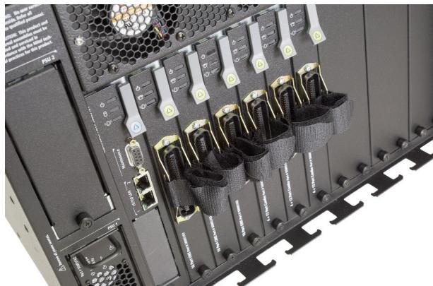
The AX Controller was designed to be an analog cabinet and can support a maximum of 250 devices, of which 192 can be analog devices. The AX Controller has capacity for 12 analog cards, as can be seen above.
