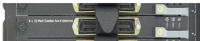
The combo card has 12 protected ONS ports and four LS trunk ports. This means analog connections to the public network can be used on the same card as a lower density of analog extensions. In the event of a power failure, the four LS trunks switch across to the first four ONS ports, creating external telephony access for any emergency situation.
