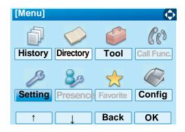
STEP 3: Select 3 Data Backup/Restore and then press (Enter) (Right-cursor) or OK soft key. (or press 3) key.)
