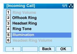
Select 1 External Call when setting the illumination pattern for external calls. Select 2 Internal Call when setting the illumination pattern for internal call. Then, press ((Enter)) or OK soft key.
