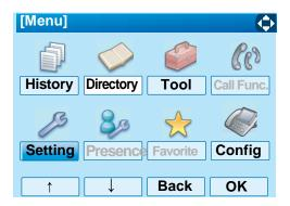
Select ① User Setting and then press ⑥ (Enter), ⑥ (Right-cursor) or OK soft key. (or press ① key.)
