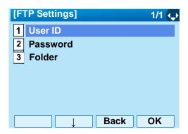
STEP 9: Enter a User ID by using digit keys, then press (Enter) or **OK** soft key.
